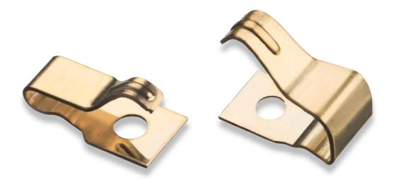
A development of the 'C' style contact, this design uses a more obvious cantilever style. The SMT pick and place area is exaggerated to compensate for the miniature size of the contact. This range is provided in 0.5mm incremental step heights, from 2mm up to 5mm. The footprint is the same across the complete set of contacts.
