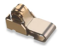
A further development of the extended 'C' style, these contacts were originally designed for wireless antenna connections on many mobile devices, such as smartphones, or LED lamp connection and RFID tags. The Positive Stop shoulder prevents the contact from being overcompressed, which can lead to permanent set and a reduction in spring force.
