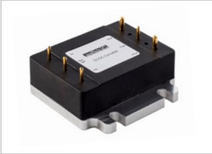
Murata's IRS Q48 & Q12 range offer an isolated single o/p, with 2250V isolation. The IRS range offers o/ps 3.3V, 5V, 12V, 15V & 24V variants. Two universal i/p ranges either 9V–36V or 18V–75V, allow for operation from 12V, 24V & 48V battery systems, including meeting the requirements of EN50155.
