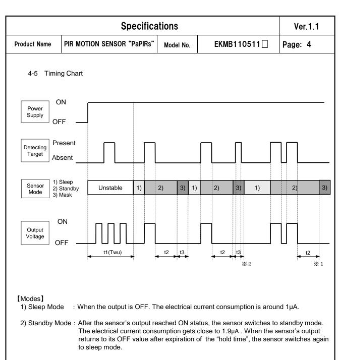
: Time during which the output is forced to OFF after the end of the standby mode. 3) Mask Mode (no detection is possible during this period.)
