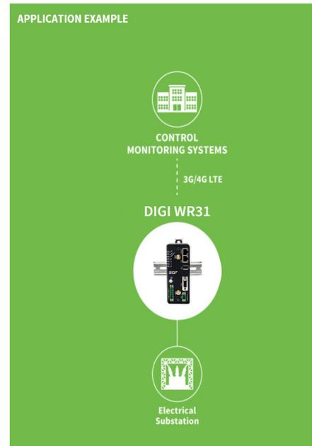
COMMUNICATION DEVICES FOR REMOTE SUBSTATION EQUIPMENT, SCADA, RECLOSERS, CAPACITOR BANKS AND OTHER TRANSMISSION EQUIPMENT
