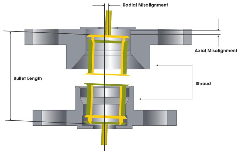
**Figure 3: RF Connector alignment**
