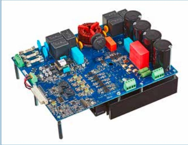
CoolSiC™ MOSFET Evaluation Board for 7.5 kW Motor Drive Applications
