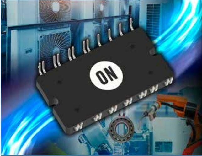
TMPIM26, a DIP-26 Transfer-Molded Power Integrated Module
