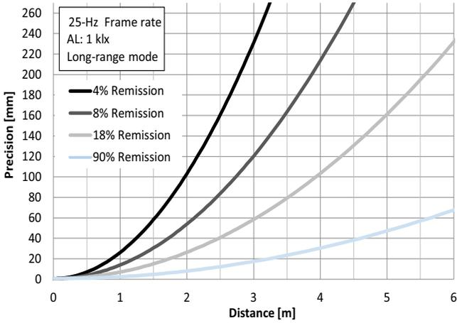
**Figure 15: Typical Precision [mm] over Distance [m] – 10 klx, Long-Range Mode**
