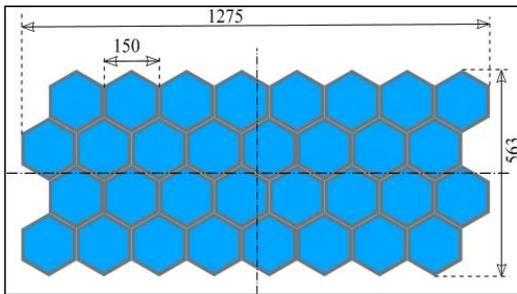
**Figure 6: Field-of-View (FoV) Description of the Sensor**
