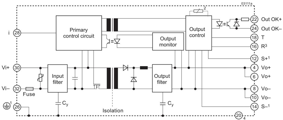
Fig. 6 1 Leading pins 2 Potentiometer for option P 3 Do not connect for models xQ1101 or with option P 4 Do not connect
