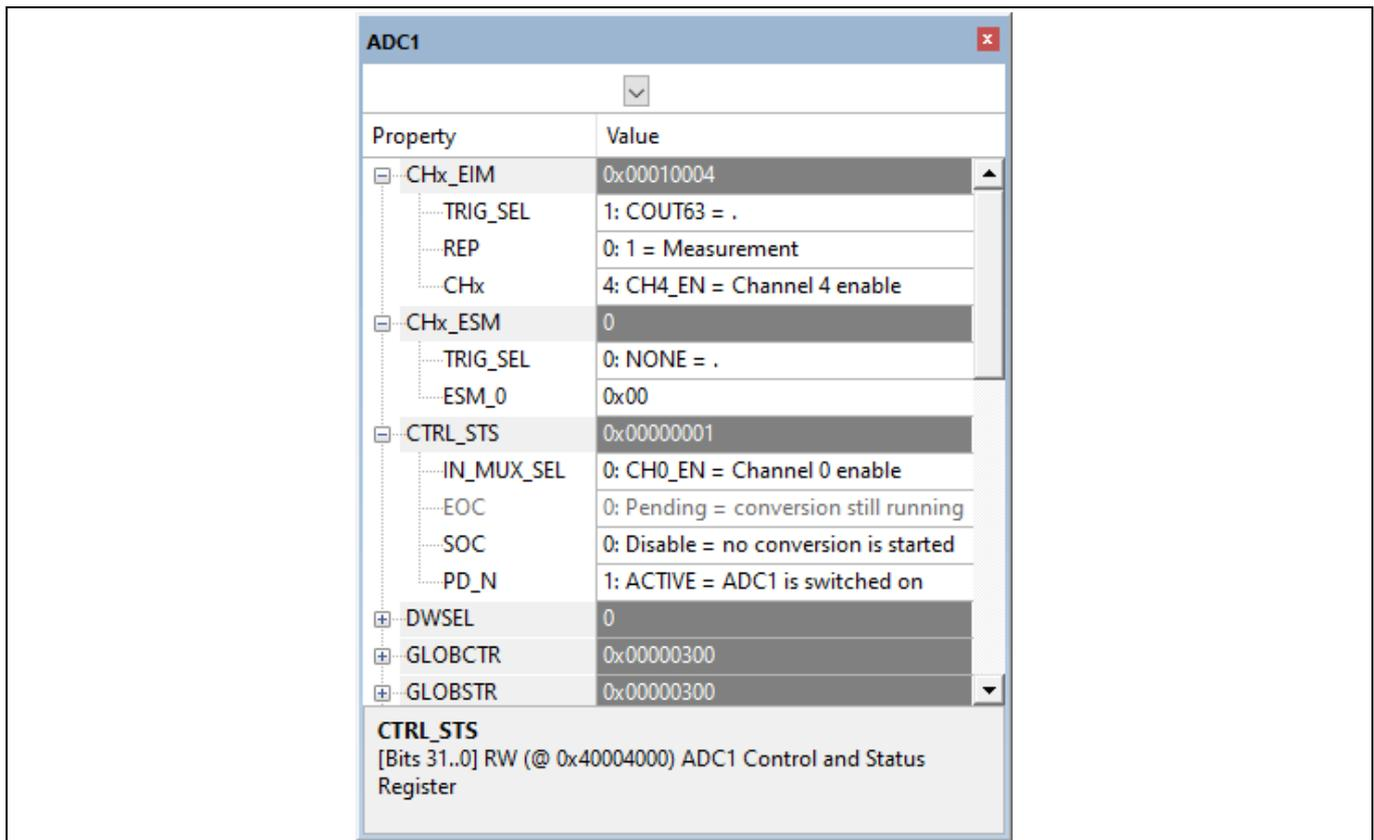
Figure 12 Registers for ADC1 module in Keil uVision
