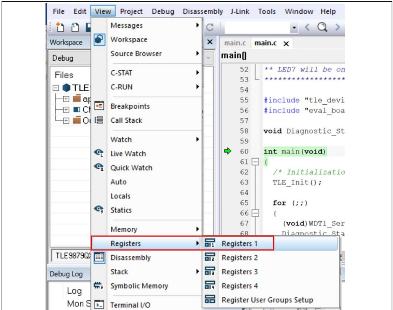
Figure 19 Register view in IAR Embedded Workbench
