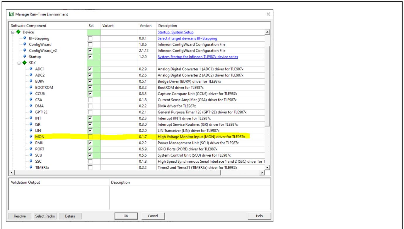
**Figure 49 Module MON is not enabled in the RTE**
