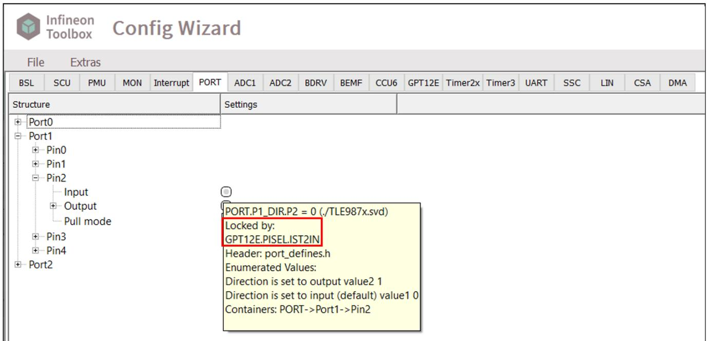
**Figure 25 Locked element in the Config Wizard**
