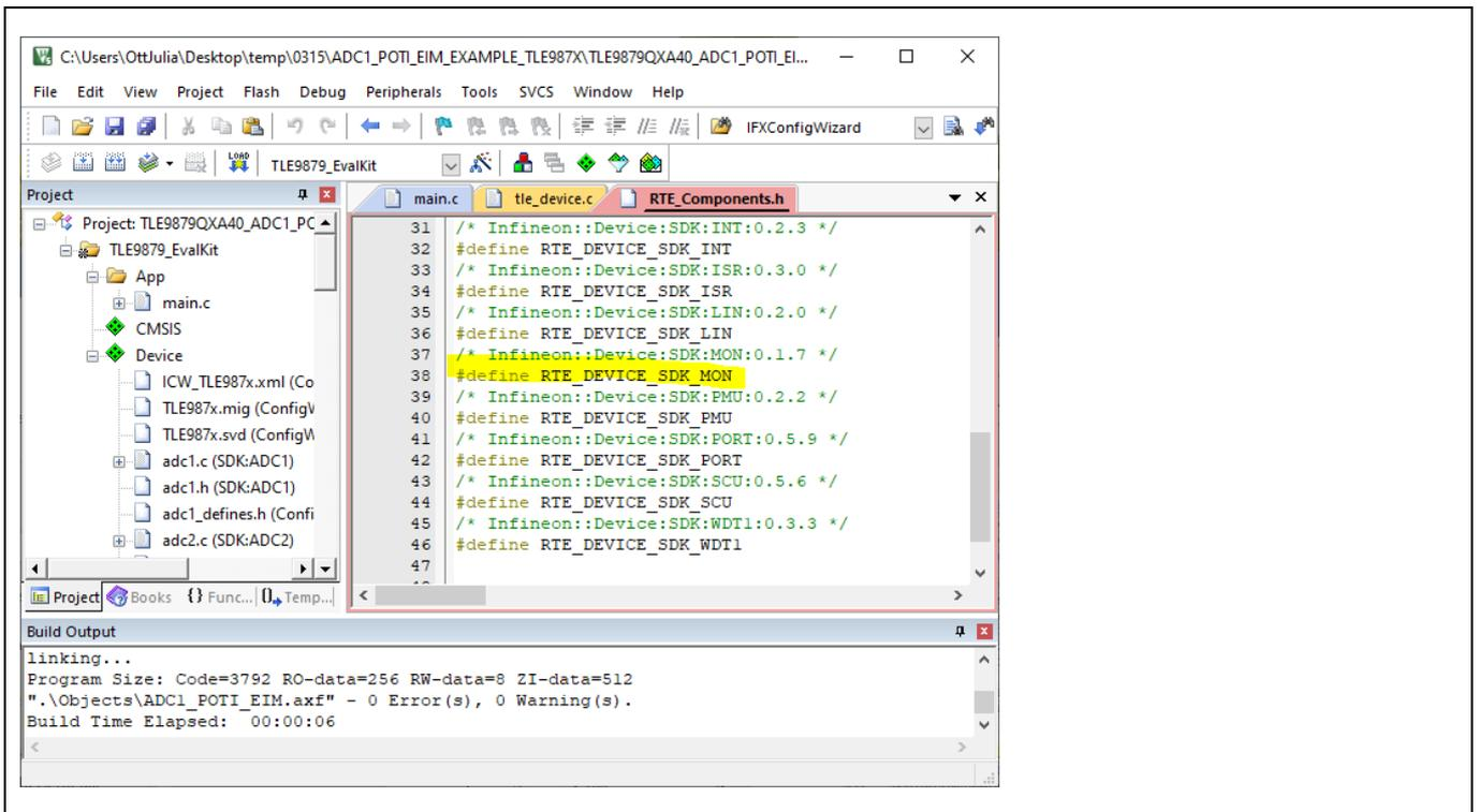
Figure 52 RTE\_DEVICE\_SDK\_MON defined in RTE\_Components.h
