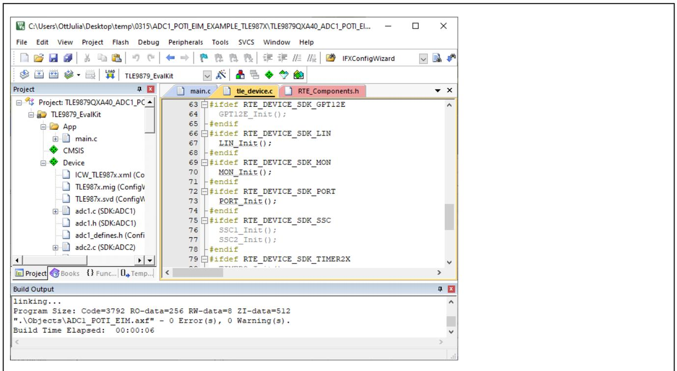
**Figure 53** Calling of a module init function in TLE\_init() is executed because RTE\_DEVICE\_SDK\_MON is defined
