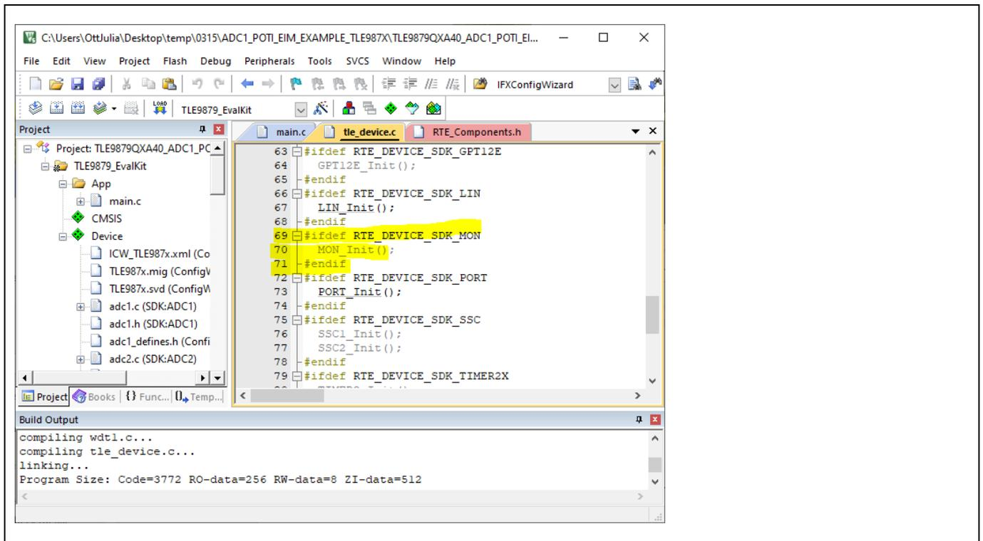
**Figure 50 RTE\_DEVICE\_SDK\_MON not defined because the module is not enabled in RTE → MON\_Init not called**
