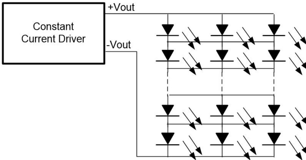
A matrix configuration is similar to a parallel configuration but extra connections are used to help minimize the effects of individual LED failures. Multiple LEDs are connected in parallel and then stacked in series. The total voltage and current would remain unchanged from the parallel configuration. If any LED fails short would cause the row of LED to stop operating while the remaining LEDs would be unaffected. Current sharing is directly related to the matching of the LEDs.
