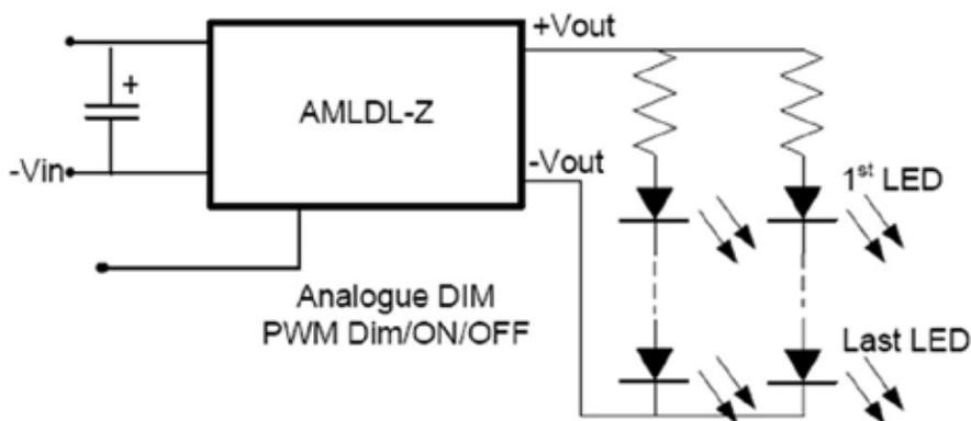
If any LED fails open all LEDs in that string will stop operating, while the other strings will continue operating. If any LED fails short, that string will carry higher current than the other strings increasing the stress levels of the remaining LEDs.
