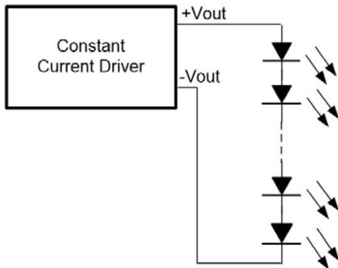
With this configuration a single constant current driver illuminates the entire string of LEDs.
