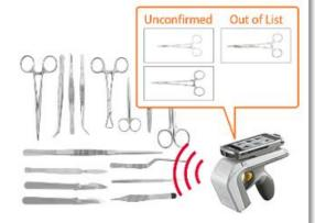
Wireless technology allows for efficient batch reading to verify each tool status
