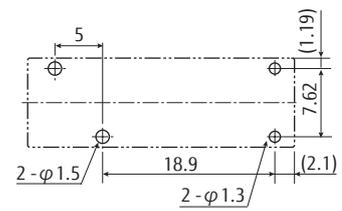
\* Tolerance of PC board mounting hole layout:  $\pm 0.1$  unless otherwise specified.
