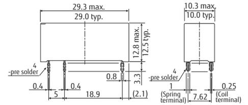
\* Dimensions of the terminals do not include thickness of pre-solder.
