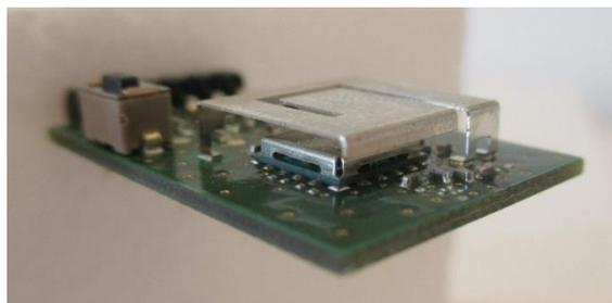
Figure 3 PIFA with RF-module and other components underneath.
