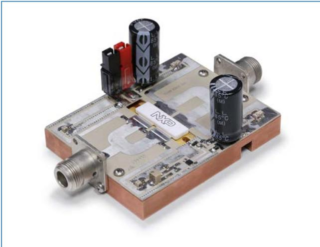
MRF13750H 915 MHz reference circuit
