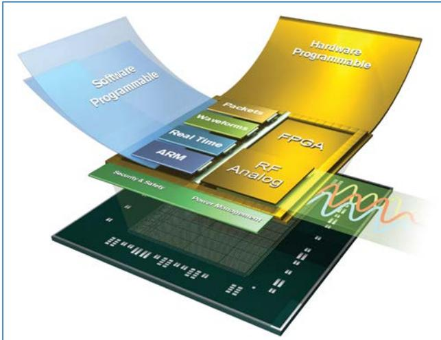
Integrating a Comprehensive RF Analog-to-Digital Signal Chain Zynq® UltraScale+™ RFSOCs integrate multi-giga-sample RF data converters and soft-decision forward error correction (SD-FEC) into an All Programmable SoC architecture.
