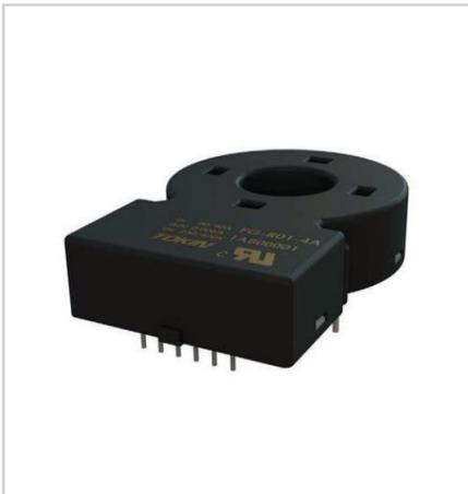
The FG-R01-4A sensor is a high-sensitivity AC and DC leakage current sensor with individual open drain alarms and an analog output for leakage current indication. In addition, its integrated test coil can be initiated by a test input to perform a functional alarm test.
