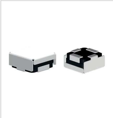
Vishay/Dale IHLE® high current inductors are AEC-Q200 qualified devices with integrated e-field shields that negate the need for separate shielding. The IHLE series is rated for temperatures up to +155°C. These inductors offer excellent DC-DC energy storage up to 2MHz and 20dB e-field reduction at 1cm. Vishay/Dale IHLE® High Current Inductors withstand high transient current spikes without saturation.
