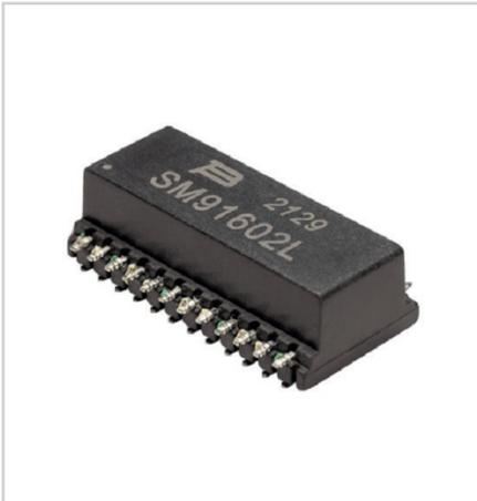
Bourns Magnetics product line introduces the model SM91602L LAN gigabit ethernet transformer. This new single-port gigabit ethernet isolation transformer includes common mode chokes for noise rejection for Ethernet applications and is designed to meet gigabit ethernet communication requirements with reinforced insulation. The model SM91602L LAN transformer offers 4680VDC isolation voltage/500V working voltage/reinforced insulation and an extended operating temperature range of 0°C to +85°C.
