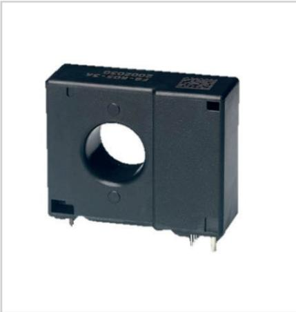
The FG-R05-3A sensor is a high-sensitivity AC and DC leakage current sensor with individual open drain alarms and an analog output for leakage current indication. In addition, its integrated test coil can be initiated by a test input to perform a functional alarm test.
