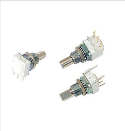
Our latest modular panel potentiometer delivers industry-high rotational torque of 8Ncm – 200 % higher than the closest competing device – in a compact 12.5mm size with a 6.35mm shaft diameter.
