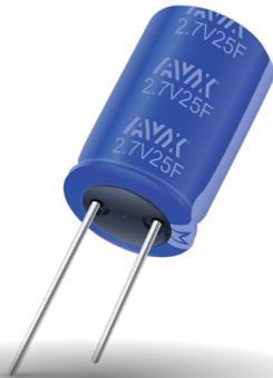
The new series of cylindrical electrochemical double-layer capacitors offers excellent pulse power handling characteristics based on the combination of very high capacitance and very low ESR. Used by themselves or in conjunction with primary or secondary batteries, they provide extended back up time, longer battery life, and provide instantaneous power pulses as needed. Offers great solutions to Hold Up, Energy Harvesting, and Pulse Power Applications.
