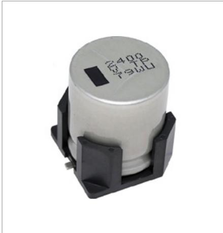
Panasonic has a line extensions for its series of electrolytic capacitors. The vibration type SMD capacitors are resistant to 30G of vibration and are available in sizes Ø6.3 – 18 (except for the EB series). Potting and adhesive fixation has been reduced in order to simplify customers' manufacturing processes.
