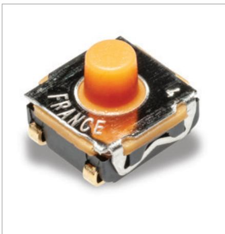
The C&K KSC DCT series offers sealed tactile switches for SMT with SPDT function. This dual-circuit functionality provides two outputs from a single input. Housed in a tiny 6.2mm x 6.2mm x 2.9mm PCB-mount package, the silicone 70SH actuator included in the package extends the height to 5.2mm above the PCB surface for easy operation and easier integration through pre/post travel.
