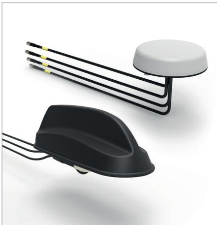
The TE Connectivity multi function MiMo antenna delivers connectivity for GSM (up to LTE), global positioning (compatible with GPS, Glonass, Galileo, and Beidou standards) and Wi-Fi connectivity in a robust housing. Designed for outdoor use, the antenna is compliant to IP66 and even protects against washing system water jets. It also withstands direct sunlight.
