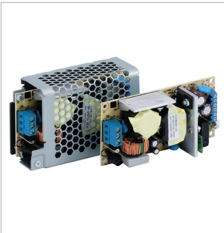
The Delta PJU series open frame power supply comes with integrated DC-UPS function. The PJU-60W, is designed to operate with an external 12VDC or 24VDC SLA battery. They will switch over to battery mode operation (batteries not included) seamlessly to prevent system downtime in the event of power disruption or unexpected loss of AC input power. The diagnostic monitoring signals available in this series, for AC OK and battery low status can alert the user.
