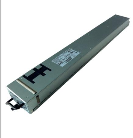
Bel Power Solutions' platinum efficiency PFE3600 series power supply, which delivers more power in a standard form factor for big data and cloud computing applications. This power supply features a compact form factor (69 x 42 x 555mm) which converts standard AC mains power or high voltage DC bus voltages into a main output of 12VDC.
