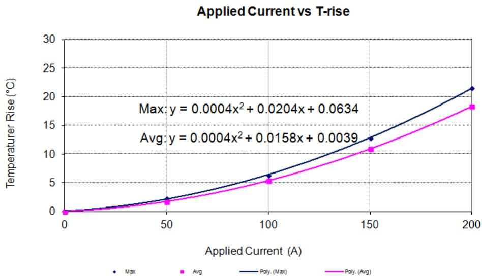
Above rating is for reference only. Appropriate de-rating is required per ambient conditions, bus bar size to achieve thermal balance, gross heating from adjacent components, and other factors that influence connector performance.
