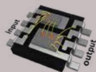
Galvanically isolated EiceDRIVER™ ICs based on our coreless transformer (CT) technology which uses semiconductor manufacturing processes to integrate an on-chip transformer consisting of metal spirals and silicon oxide insulation. The on-chip transformers are used for transmitting switching information between input chip and output chip which are galvanically isolated.
