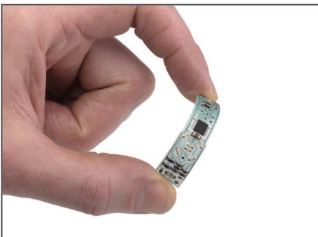
**Figure 2:** Depending on the complexity of a printed sensor design and its intended function, transitioning from an FR-4 circuit board to printed silver on a lower cost polymer substrate may be the best option.
