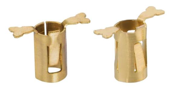
Previous designs of SMT contacts have only included 2 points of contact to the mating pin, making them potentially vulnerable to vibration. The <u>Sycamore</u> <u>Contact</u> patent-pending design incorporates 3 points of contact for improved continuous signal integrity.
