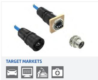
Amphenol's IP67 rated SPE connectors have a circular M12 size form factor with push-pull positive latching. Robust panel-mount receptacles are available with right angle and vertical PCB tails or solder cups for discrete wire termination. When mated with the field terminable plugs, a completely sealed, shielded interface is provided, rated up to 4A supporting PoDL (Power over Data Link) up to 1km when using 18AWG single pair cable.
