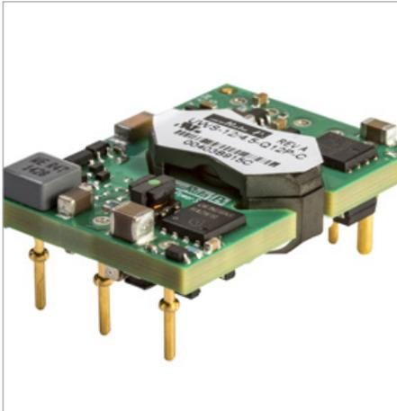
The world of brick DC-DC converters has seen a steady size reduction. The UWS-Q12 series makes another dramatic size shrink down to a sixteenth brick width while still retaining a high power output and full 2250VDC I/O isolation. The converter family accepts 9VDC to 36VDC inputs and delivers fixed regulated outputs. The UWS converters are ideal for mobile applications, datacom and telecom applications, cell phone towers, data centers, server farms and network repeaters.
