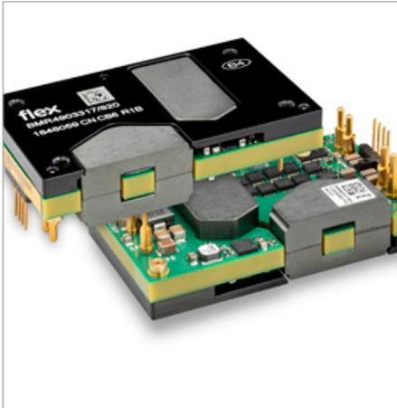
Flex has launched the BMR490, a non-isolated digital IBC (Intermediate Bus Converter) DC-DC converter with an output power of 1300W in the quarter-brick form factor. The converter combines very high power density with excellent thermal performance in a price-sensitive design, making it ideal for demanding applications such as data centres.
