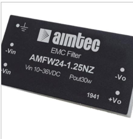
Aimtec's EMC filter modules are extremely useful in reducing noise in sensitive analog circuit applications. Filters connected on the input of DC-DC converters can ensure system compliance with EMC requirements according to IEC/EN61000-4 and CISPR32/EN55032 standards. Aimtec's DC-DC converter modules can be paired with the new generation of Aimtec's EMC filters to achieve the required compliance. The Aimtec EMC line can currently offers solutions up to 30W output power.
