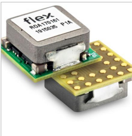
The Flex's PNA converter is an analog device with a small form factor 12mm x 12mm x 6.5mm and delivers up to 6A. The main application area is the industrial sector due to its input voltage range of 9V to 32V. The output voltage range is 0.9V to 5.5V. The PNA converter has max. power of 33W and the efficiency lies at 89.7% at 24 Vin and 3.3 Vout.
