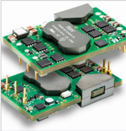
The PKM-NH series power modules are fully regulated DC-DC converters, offering extreme high power 864W in a quarter brick size, using advanced regulation for high power efficiency, high current double output pinning together with evolved thermal management, which makes this series products very suitable for a wide range of demanding applications.
