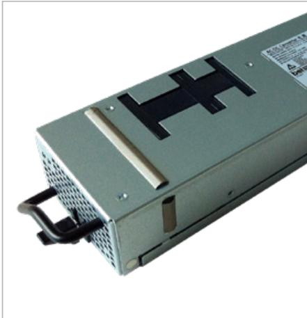
The PFE3000 series is a 3000W AC-DC Power-Factor-Corrected (PFC) and DC-DC power supply that converts standard AC mains power or high voltage DC bus voltages into a single main output of either 12VDC for powering Intermediate Bus Architectures (IBA) in high performance and reliability servers, routers, and network switches or 360VDC for powering high voltage DC equipment.
