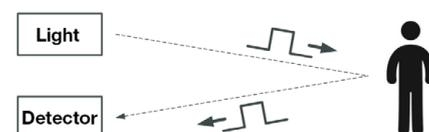
Schematic representation of ToF technology: Light is emitted (diode), this hits an object (person), the light is reflected and then detected in the sensor. The distance of the object to the sensor can then be determined from this data.
