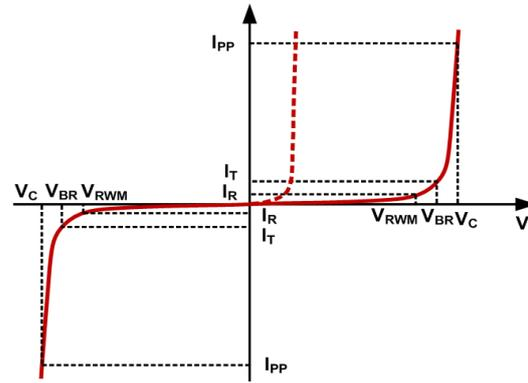
Figure 6. TVS Characteristic Curve and Parameter Description
