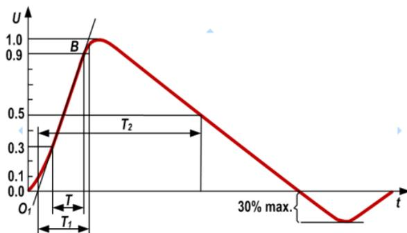
Figure 1. 1.2/50μs Voltage Waveform
