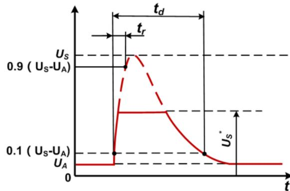
Figure 4. Load Dump 5a/5b Waveform
