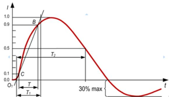
Figure 2. 8/20μs Current Waveform
