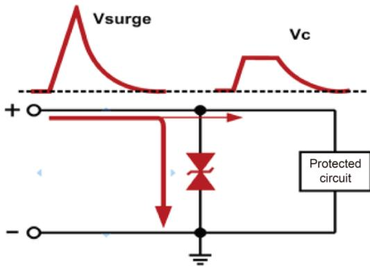
Figure 5. Diagram of Surge Absorption
