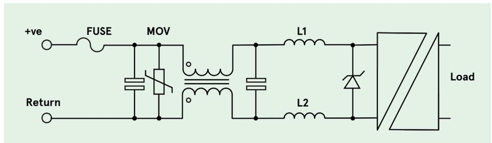
Figure 6: Common mode noise filtering
