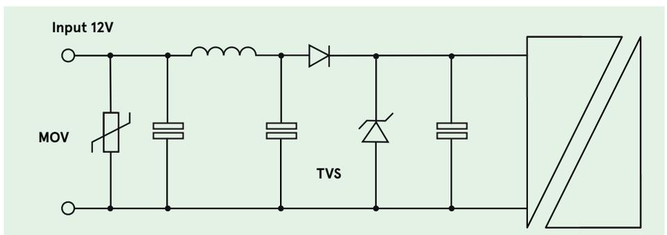
Figure 3: Automotive DC-DC input filter
