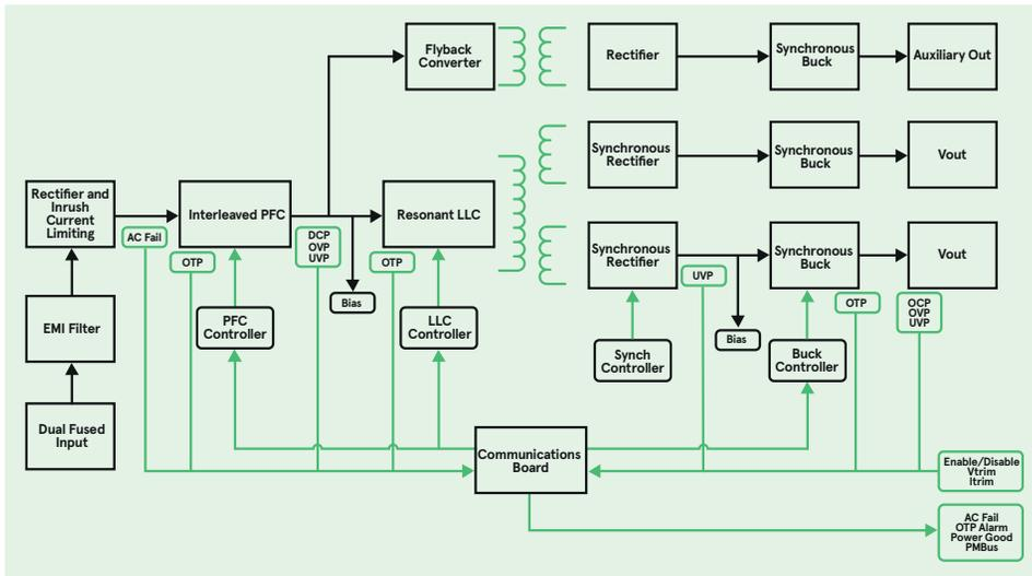
Figure 1: Typical configurable power supply architecture
