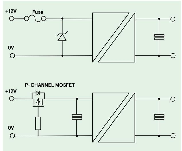
Figure 4: Reverse polarity protection options
