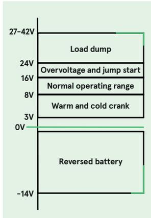
Figure 2: Summary of 12V DC-DC converter input range requirements
