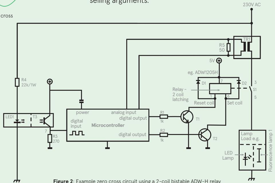
Figure 2: Example zero cross circuit using a 2-coil bistable ADW-H relay
