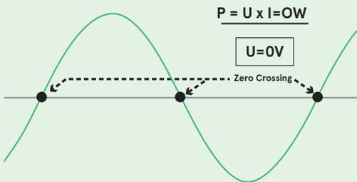
Figure 1: Switching the relay at the zero cross
