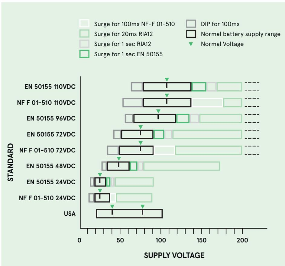
Figure 5: Input voltage ranges for rail applications
