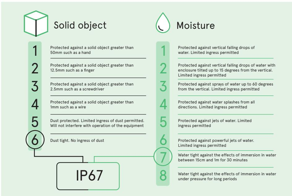
Figure 2: Ingress Protection (IP) ratings
