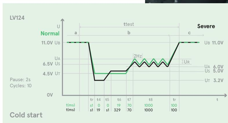
Figure 1: LV124 cold cranking conditions
