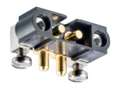
Mix-Tek uses the same outer housing design as J-Tek, with each power contact taking up the space of 4 signal contacts (giving 4mm pitch). The original power contacts are capable of up to 20A, and the latest High Power contacts will carry 40A each.
