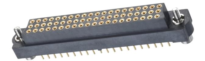
Datamate connectors are all based on a 2mm pitch system, with contact counts from 2 to 96. This compact system gives improved current rating over classic 2mm pitch pin header and socket systems, as well as meeting the high-reliability requirements with the vibration and temperature specifications.
