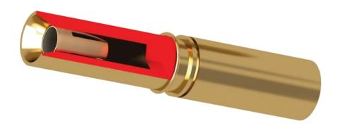
A 4-fingered Beryllium Copper female contact gives superb performance, for both electrical and mechanical specifications. This inner "contact clip" is stamped and plated with a durable gold finish at our UK headquarters. The spring performance of the contact gives the environmental resistance to shock and vibration, with a temperature range up to 125 degrees C.
