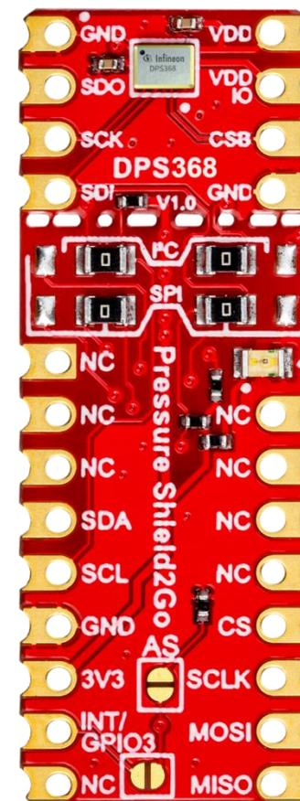
Ensure that no voltage applied to any of the pins exceeds the absolute maximum rating of 4 V
