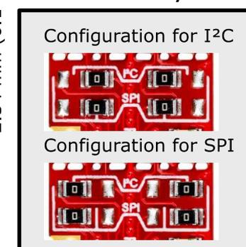
**i** The board can be switched from I<sup>2</sup>C mode to SPI mode by moving 0 Ohm resistors.
