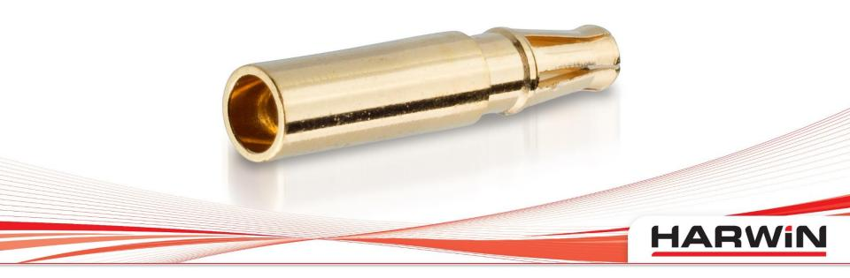
The T-Contact is only available in a gold-plated finish. To maximise durability, the gold is applied at 0.76- $1.00\mu m$  (30- $40\mu''$ ) thickness, over nickel & copper undercoats. This improves the durability from the existing 500 mating cycles to 1,000 mating cycles without degradation. This meets the more demanding standards of the military and aerospace requirements.
