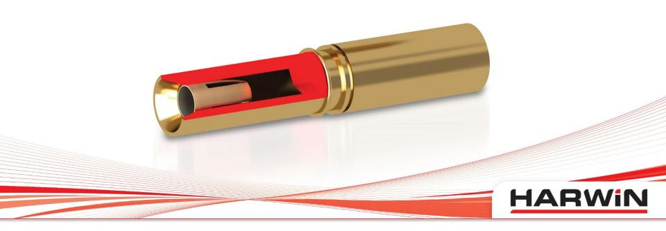
The current signal contact used on all Datamate variations is constructed from a 4-fingered Beryllium Copper female contact clip, housed inside a brass turned shell. The contact system gives superb performance, for both electrical and mechanical specifications, with environmental resistance to shock and vibration, and a temperature range up to 125 degrees C.
