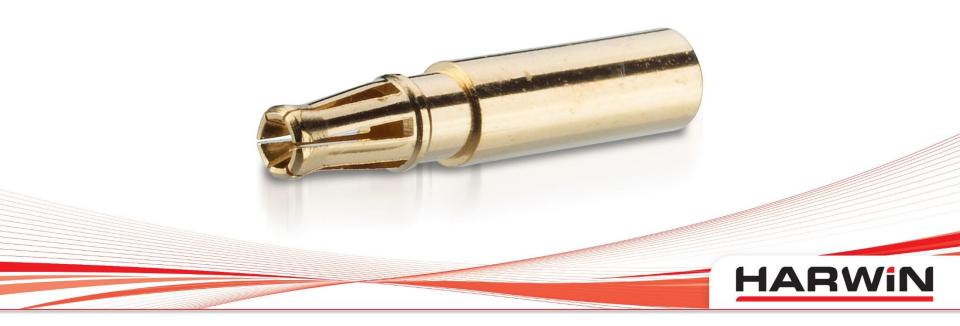
The T-contact is an advanced design, based on the research around the Gecko connector system. By using a single piece of Beryllium Copper in a turned design, the current-carrying capacity of the contact is improved, due to additional mass of metal. Beryllium Copper is used as the base metal to ensure the spring qualities of the contact area are maintained.
