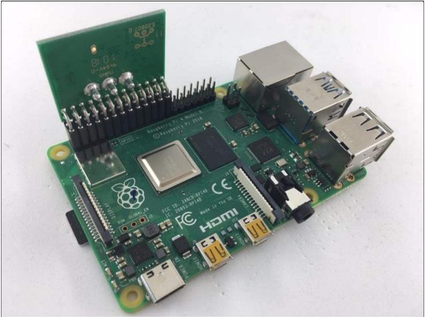
**Figure 2 Infineon Iridium SLx 9670 TPM2.0 SPI Board on Raspberry Pi® 4**
