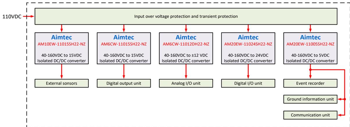
Figure 6. Train operation monitor system
