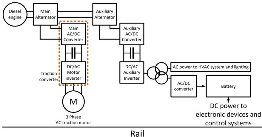
Depending on the manufacturers, the train auxiliary power voltage level can be either 24V, 36V, 48V, 72V, 96V or 110V. 110V and 72V are the most common voltage levels as higher voltages lower the current and reduce the wiring space and weight. However, most of the electronic devices require 3.3V, 5V or 12V. This is where the Aimtec railway power supplies can step in and help to convert the higher auxiliary voltage into one that can power the electronic devices.
