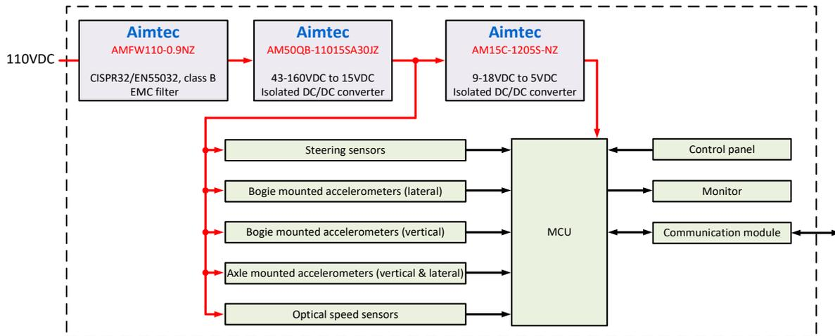
Figure 4. Bogie monitoring system
