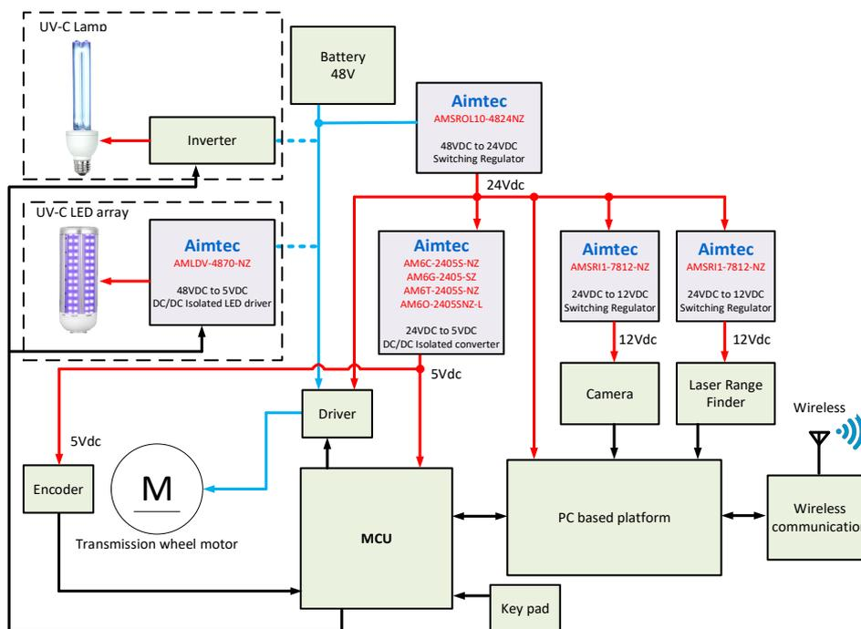
Figure 9. UV-C disinfection robot
