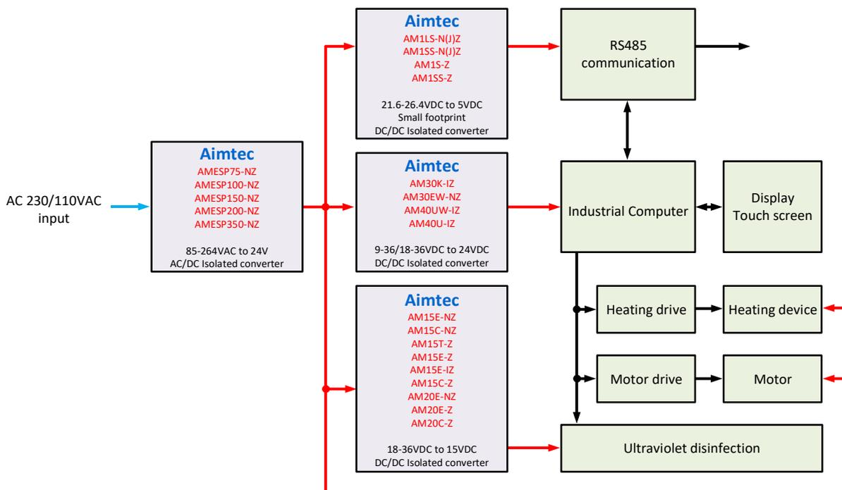
Figure 1. Automatic nucleic acid extraction instrument
