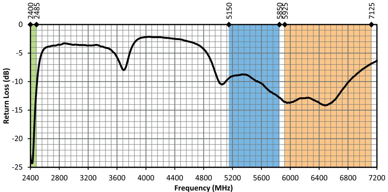
Figure 5. ANT-W63-CW-RCS-ccc Return Loss, Free Space
