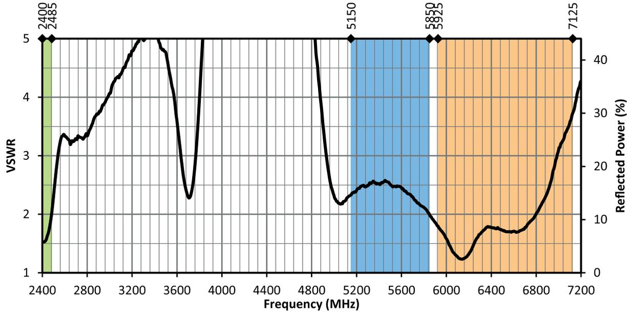
Figure 11. ANT-W63-CW-RCS-ccc VSWR, on Edge of Ground Plane
