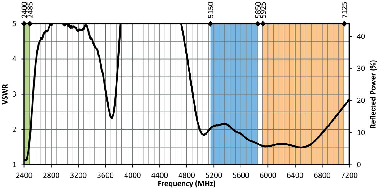
Figure 4. ANT-W63-CW-RCS-ccc Antenna VSWR, Free Space
