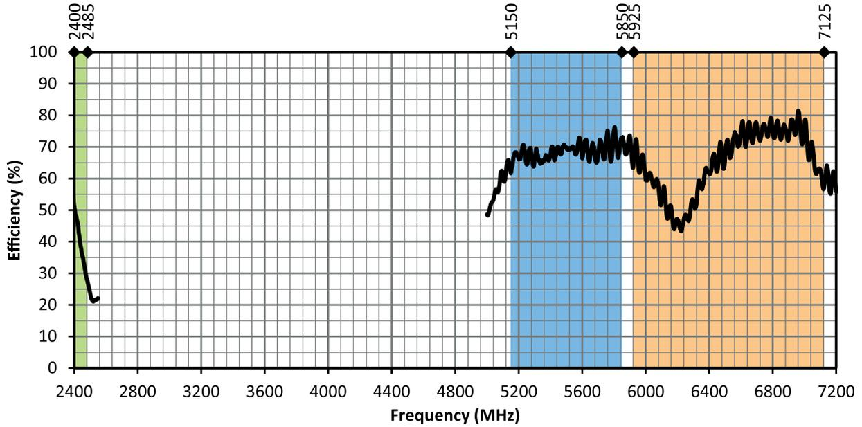
Figure 8. ANT-W63-CW-RCS-ccc Antenna Radiation Efficiency, Free Space
