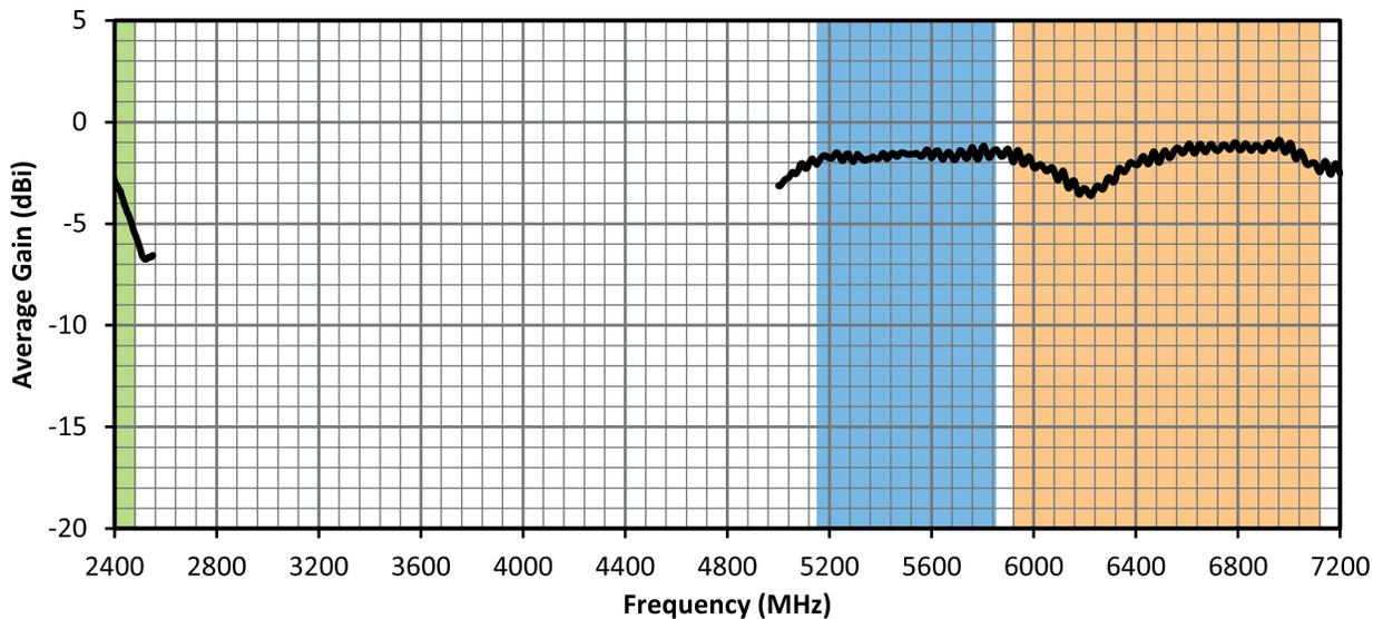
Figure 7. ANT-W63-CW-RCS-ccc Antenna Average Gain, Free Space
