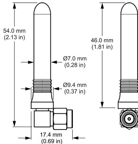
Figure 1. ANT-W63-CW-RCS-ccc Antenna Dimensions
