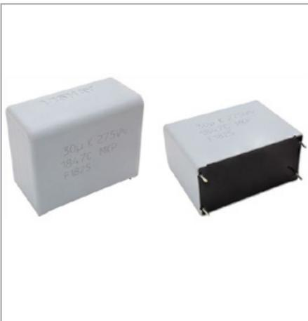
Vishay Intertechnology series of metallised polypropylene AC filtering film capacitors is optimised for high humidity environments. Vishay Roederstein MKP1847C AC filtering devices withstand demanding Temperature Humidity Bias (THB) testing –40°C, 93% relative humidity for 56 days at rated voltage without altering their electrical characteristics.
