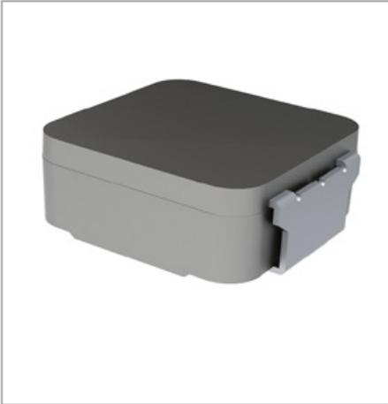
The KEMET MPEV metal composite inductors are ideal for use in DC-DC switching power supplies for automotive applications. The metal composite core has high saturation characteristics maintaining functionality with high current transients and is characterised by temperature stable inductance. The high heat resistance propriety of the inductor has been further improved and allows for operating temperature up to +180°C.
