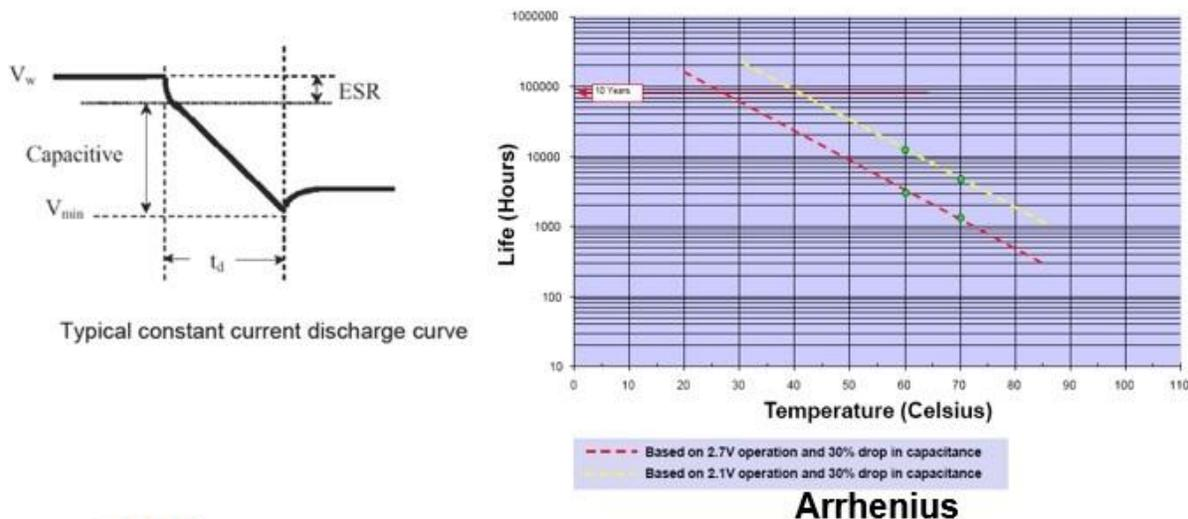
**Figure 1 - When sizing supercapacitors, consider voltage drops due to initial current pulse (ESR) and life/aging due to time, voltage, and temperature, as shown in the Arrhenius graph above.**
