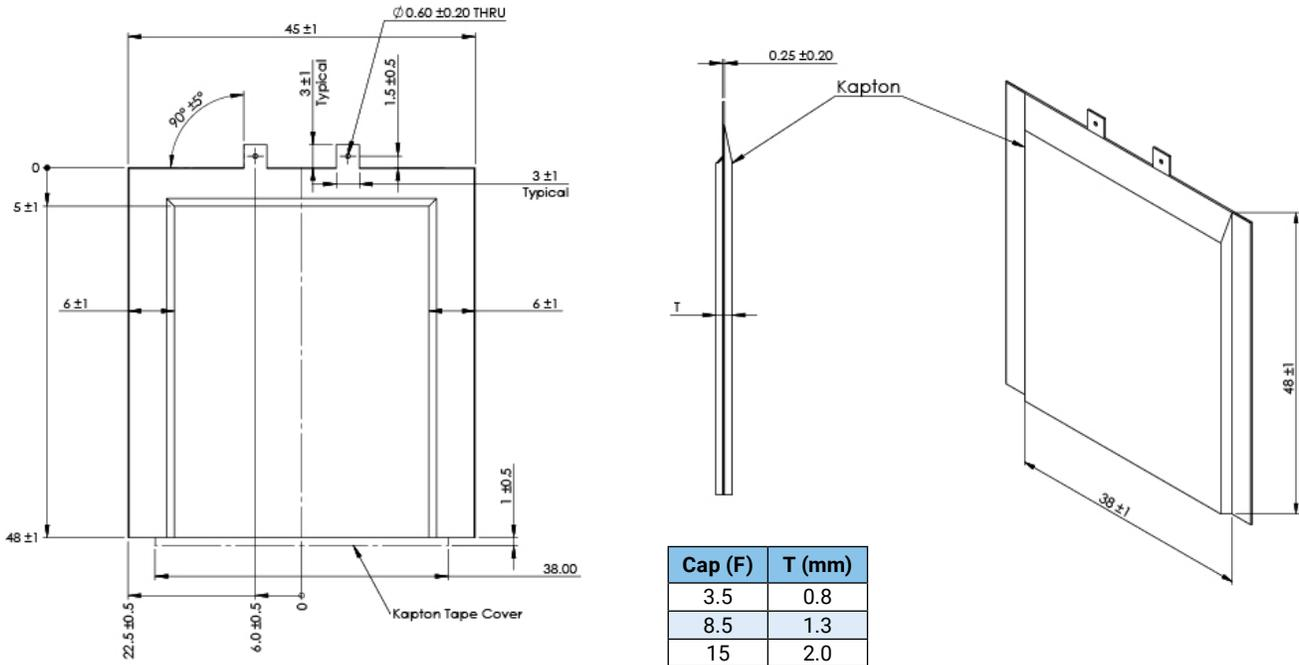
Note: When the supercapacitor is used under stressed conditions, it is expected to see some expansion of the supercapacitor. Expansion of the supercapacitor will not affect lifetime or performance.
