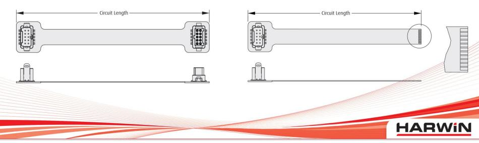
On these Flex Circuit assemblies, cable length is specified as the total length of the FPC.
