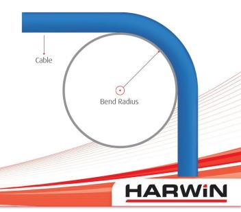
Flex circuit is able to bend at a much tighter angle than cable. Where a typical static bend radius for these flex circuits is 10 times the thickness of the flex, the thickness of the flex means this is just 1.85mm. For a 28AWG cable, the static bend radius might at best be 3.36mm (Ø0.56mm x 6), but could be 7.10mm (Ø0.71mm x 10).
