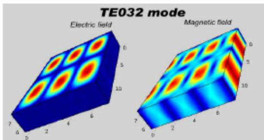
*Field distribution of TE032 mode inside an empty cavity dielectric foam absorbers*
