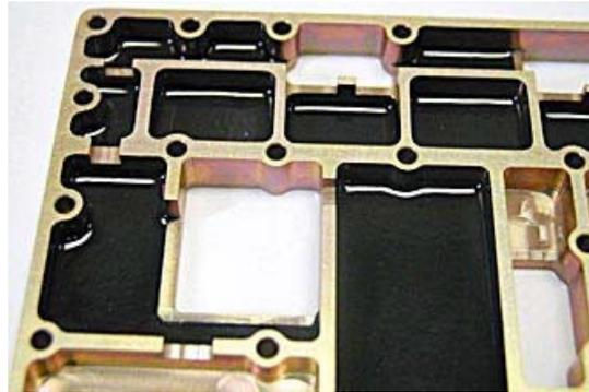
*Absorber molded in place in a circuit board cover to damp cavity resonances*
