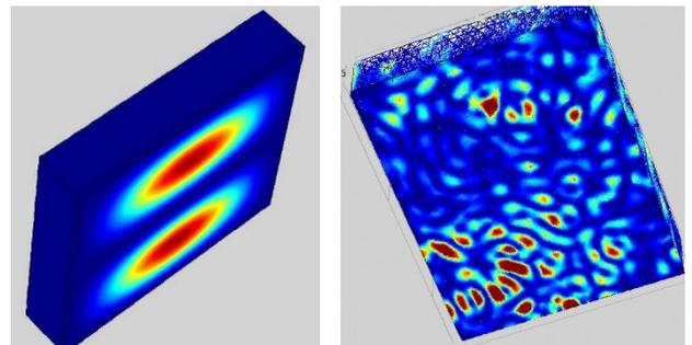
*The image on the left is the electric field distribution inside a cavity approximately 2 wavelengths in dimension. Note the clearly delineated resonance peaks indicating cavity resonance. The image on the right is the electric field distribution inside a cavity >10 wavelengths. While there appears to be some resonant behavior there are clearly some propagating elements as well.*
