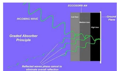
will enable the 377 ohm input impedance condition over a broader range of frequencies. The design of this class of material is similar to design for a quarter wave transformer.
