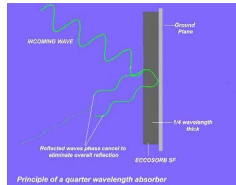
There are no separate reflections off the front and back surface. Like virtually everything else in the microwave engineering world, absorber design is an impedance matching problem, in this case matching the impedance of a metal surface ( $Z=0$ ) to the impedance of free space ( $Z=377$  ohms). If the impedance seen by the wave at the surface of the material is equal to 377 ohms, the wave will be completely absorbed by the material.
