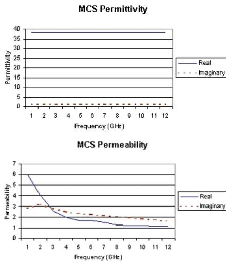
*Typical parameters for a magnetic microwave absorbent material*
