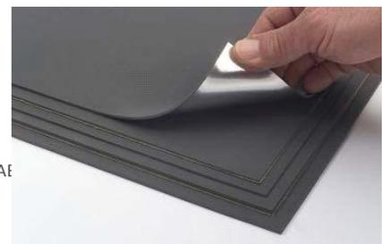
magnetic loss. Advantages include the ability to greatly compress the wavelength due to the high permeability enabling quarter wavelength resonant absorbers at a thickness that are a fraction of the free space wavelength. Also, magnetic absorbers are best for cavity resonance damping since the magnetic field is a maximum on the conductive surface where the absorber is placed. Disadvantages of magnetic absorber include weight and cost.
