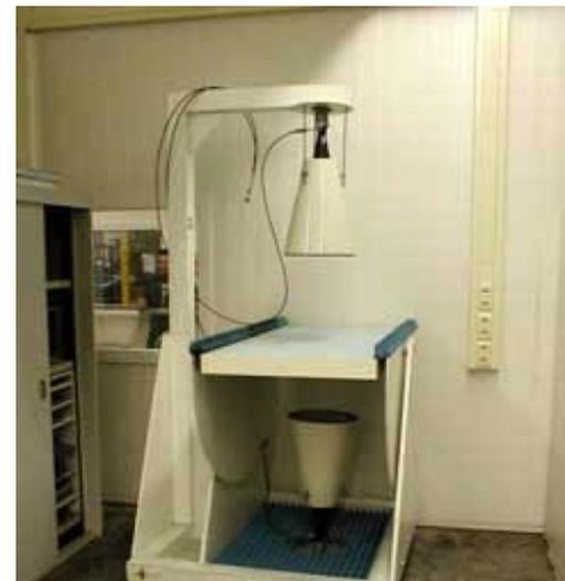
**Insertion Loss Test Setup**
