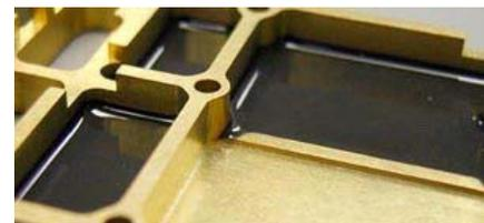
*A cavity resonance absorber molded in place inside a circuit board*
