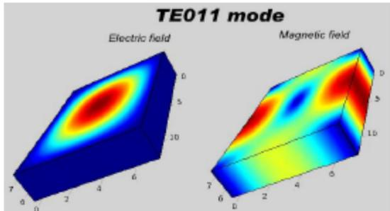
*A range Field distribution of TE011 mode inside an empty cavity*
