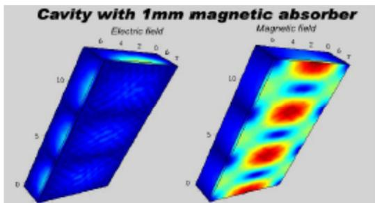
*Field distribution in cavity with magnetic absorber at 1mm thickness  $f_r=2.36$  GHz*
