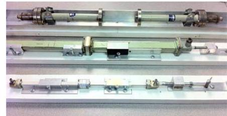
*Waveguide and coaxial test fixtures*
