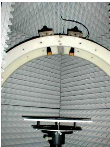
*An NRL Arch for millimeter wave measurements*
