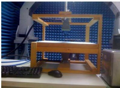
*Insertion loss/phase test fixture for broadband parameter measurement of non-magnetic material*
