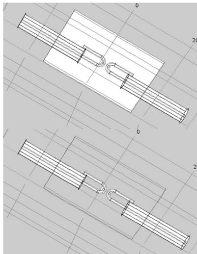
*Near field model with coupling loop antennas with and without absorber*
