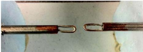
*Coupled loops for inter and intra decoupling test*
