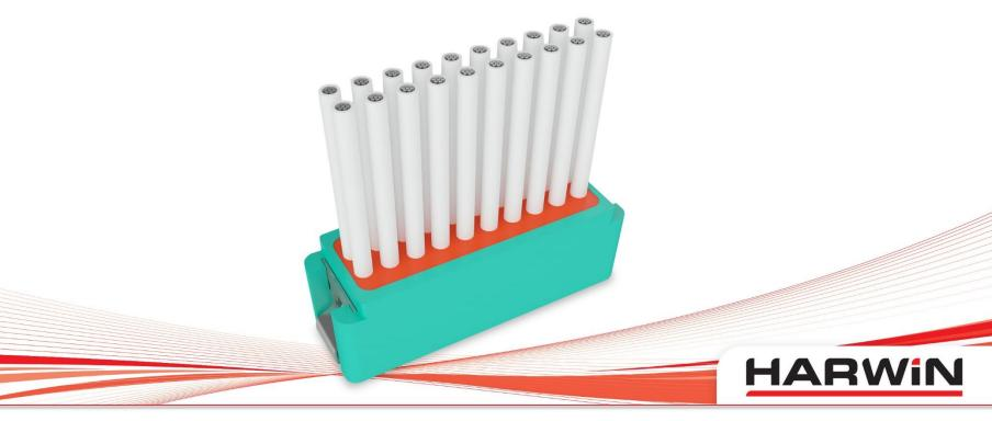
The crimp housings feature a potting wall to keep potting fluids retained during application. The use of potting improves the retention of the crimp contacts in the housing by adding strain relief. For the full connector assemblies supplied by Harwin, potting compound has already been applied.
