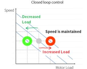
The device maintains constant rotation speed during load variation
