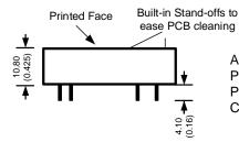
All dimensions are typical: millimeters (inches) Pin Diameter:  $0.50 \pm 0.05$  ( $0.02 \pm 0.002$ ) Pin Pitch Tolerance:  $\pm 0.35$  ( $\pm 0.014$ )
