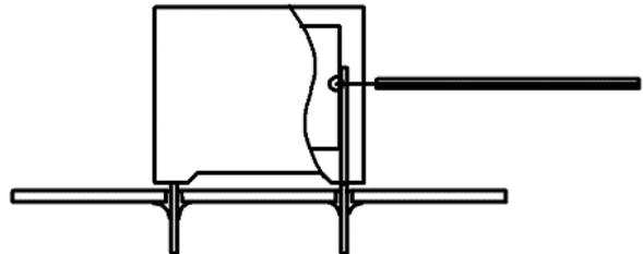
*Temperature monitored inside the capacitor.*
