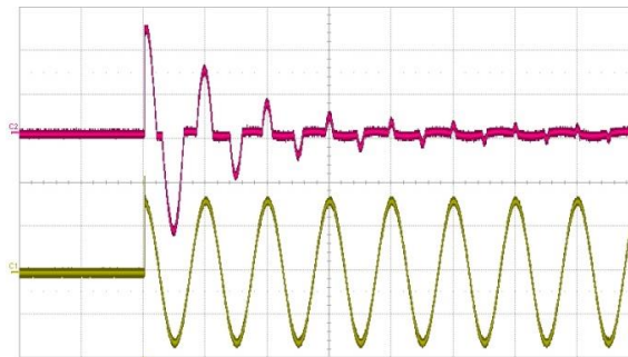
Figure 4 - Inrush current, V_{in} = 230V_{ac} , 90^\circ CH4: V_{in} (200V/div), CH2: I_{in} (5 A/div)
