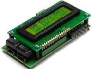
SMBus Reader                               | 100122                               | Simple read out of SMBus batteries data. No external power supply required. 5way blade connector and RS232 interface.                                                                                                           |
